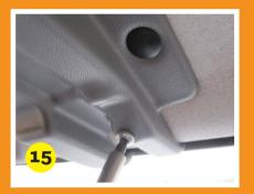
Place the sun-visor onto the outer section of the roof console. Use the longer sun-visor fixing screws
