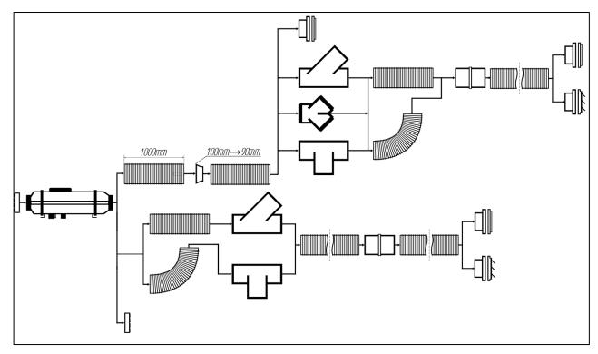
Fig. 26c – Air duct connections for AIR- 9D (100mm/90mm)
