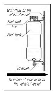
Fig. 16 Installation of the fuel tank
