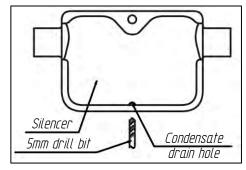
Fig. 10a – Condensate drain hole for horizontal mounting
