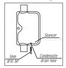
Fig. 10b – Condensate drain hole for vertical mounting
