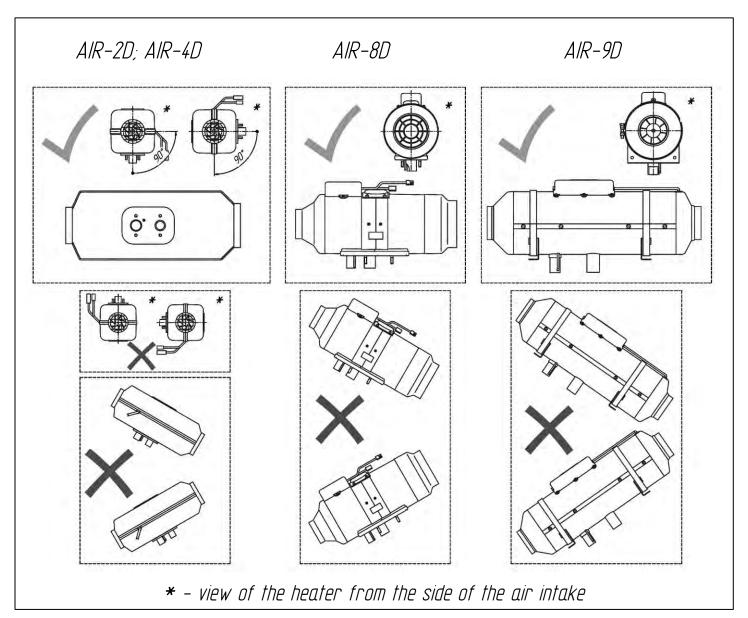
Fig. 1a - Mounting positions of the heater
