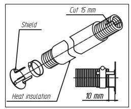
Fig. 9 – Exhaust pipe shield
