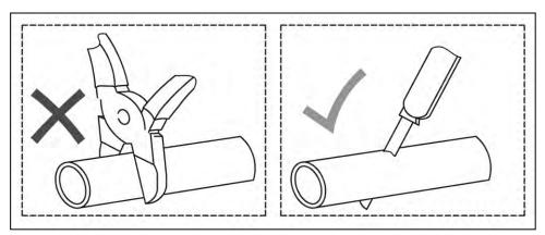
Fig. 21 - Cutting of the line before installation.
