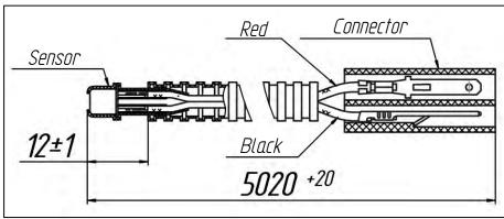
Fig. 23 - Temperature sensor
