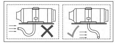
Fig. 5 – Position of air intake/exhaust pipe
