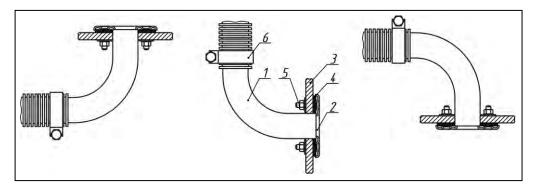
Fig. 7 - Installation of the air intake pipe
