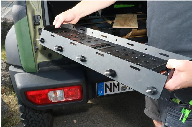
The first step is to screw the side panels and the flat plate are screwed onto the vehicle.
